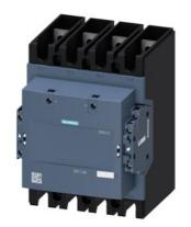
Contactor, AC-1, 350 A/400 V/40 °C, S10, 4-pole, 100-250 V AC/DC, 2 NO+2 NC, Connection rail/ screw terminal
