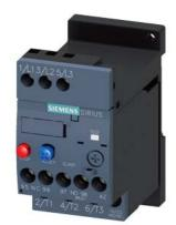
Overload relay 0.22...0.32 A Thermal For motor protection Size S00, Class 10 Stand-alone installation Main circuit: Screw Auxiliary circuit: Screw Manual-Automatic-Reset
