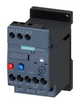
Overload relay 0.35...0.50 A Thermal For motor protection Size S00, Class 10 Stand-alone installation Main circuit: Screw Auxiliary circuit: Screw Manual-Automatic-Reset
