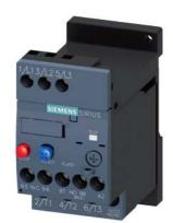
Overload relay 0.70...1.0 A Thermal For motor protection Size S00, Class 10 Stand-alone installation Main circuit: Screw Auxiliary circuit: Screw Manual-Automatic-Reset
