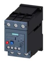
Overload relay 40... 50 A Thermal For motor protection Size S2, Class 10 Stand-alone installation Main circuit: Screw Auxiliary circuit: Screw Manual-Automatic-Reset
