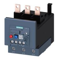
Overload relay 70...90 A Thermal For motor protection Size S3, Class 10 Contactor mounting Main circuit: Screw Auxiliary circuit: Screw Manual-Automatic-Reset
