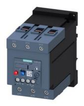
Overload relay 80...100 A Thermal For motor protection Size S3, Class 10 Stand-alone installation Main circuit: Screw Auxiliary circuit: Screw Manual-Automatic-Reset
